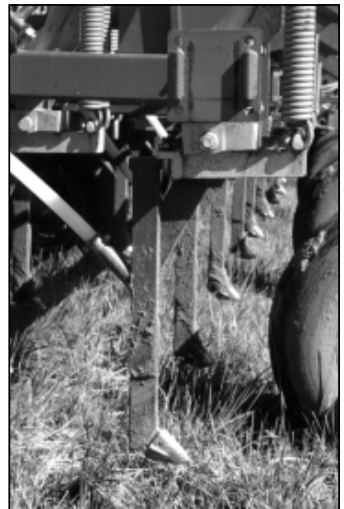
Vertical shank built by Gord and Wayne Freitag. The Gen 43 tip has 6000 acres on it.
