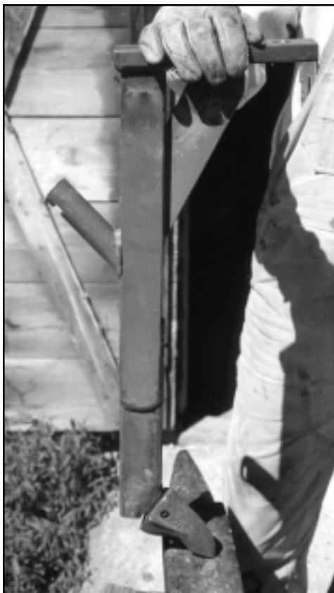
Side view of shank showing notched seed tube and new Gen 43 tip
