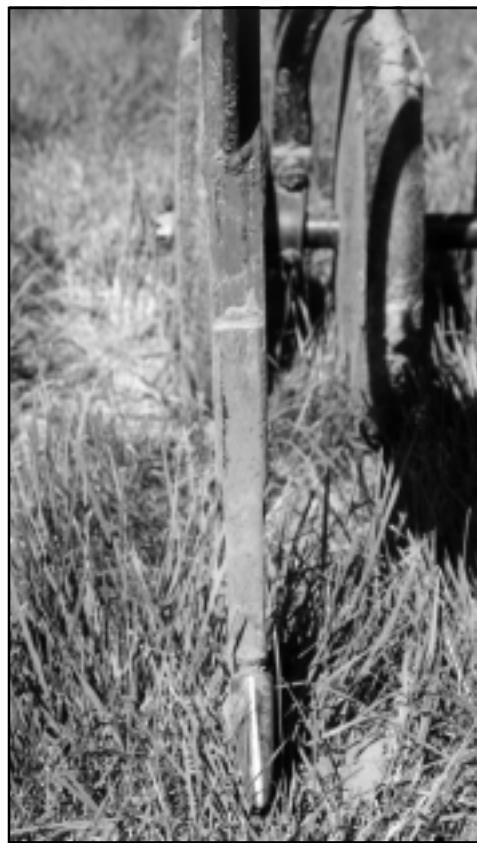
Front view of shank showing its narrow profile and front wear plate
