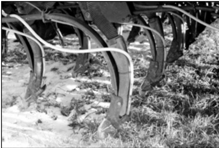
Clarke's JD 9450 hoe drill modified with K-Hart liquid MRB coulters and Gen eagle beak openers.
