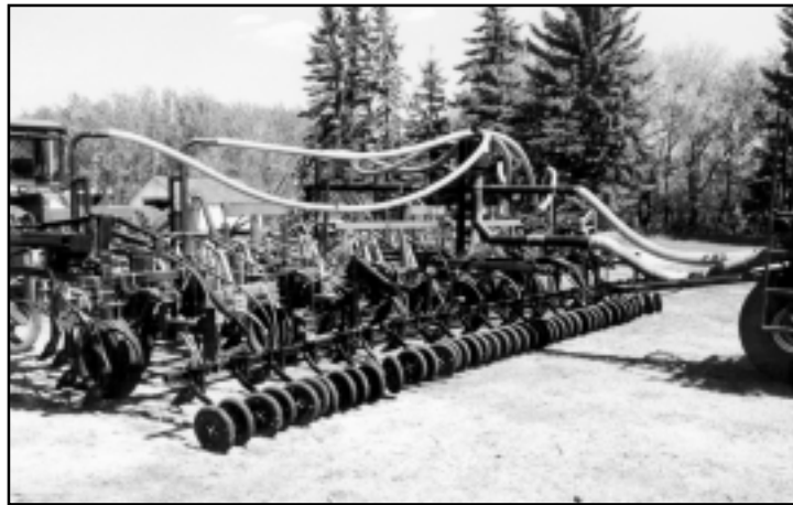
Bourgault airseeder retrofitted into a LDS system
