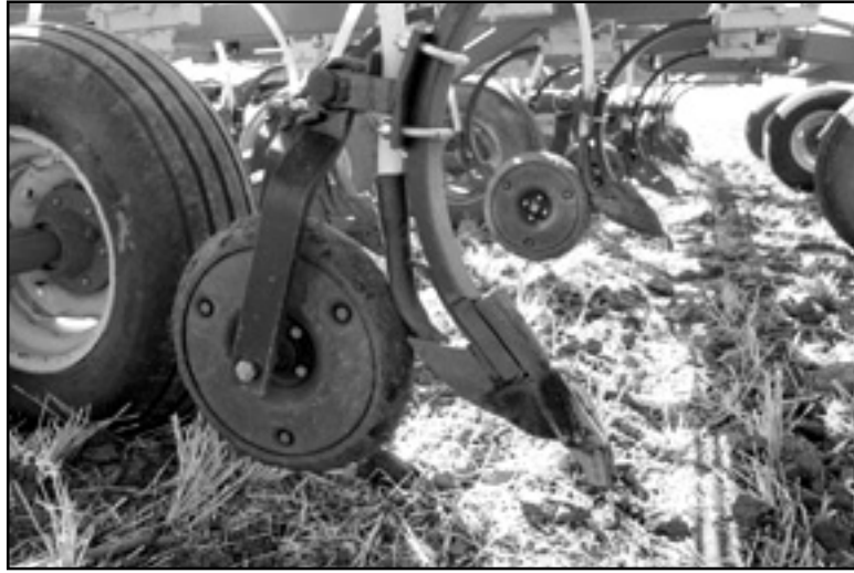
Fedak's Bourgault 8810 with Bourgault 1 inch vertical knife and Valley System's shank mounted packers.
