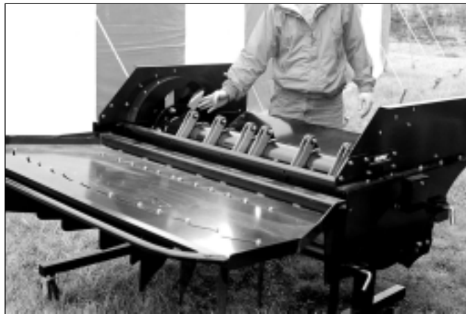
Figure 1: MAV display chopper. Notice the paddles and shroud, which direct the air for maximum spread. The spring pin that is used to quickly set tailboard position, has just recently been replaced with an optional in-cab adjustment.
