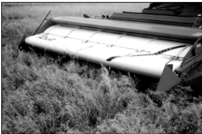
Stripper header harvesting lentils.
