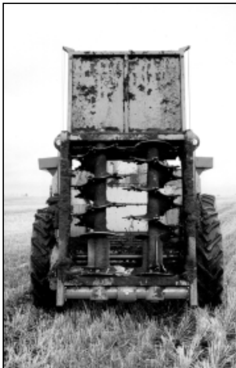
Rear view of the Bunning Lowlander Range manure spreader. PTO driven vertical beaters operate at roughly 400 revolutions per minute.
