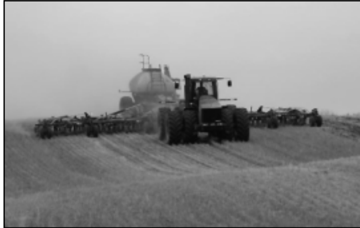
The Simpson's 57' Flexi-Coil 5000 air drill with the Flexi-Coil 50 series air cart. The air cart has three tanks and the variable rate option.
