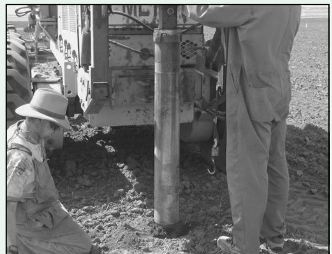
A hydraulic-powered grader was used to place lysimeters (i.e., tubes) into the 120 cm depth of the soil before a crop was seeded into the lysimeter.
