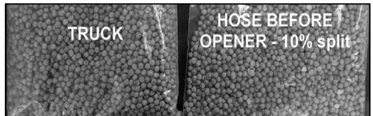
Fig. 2. Damage to the pea seed that can happen during the seeding operation.
