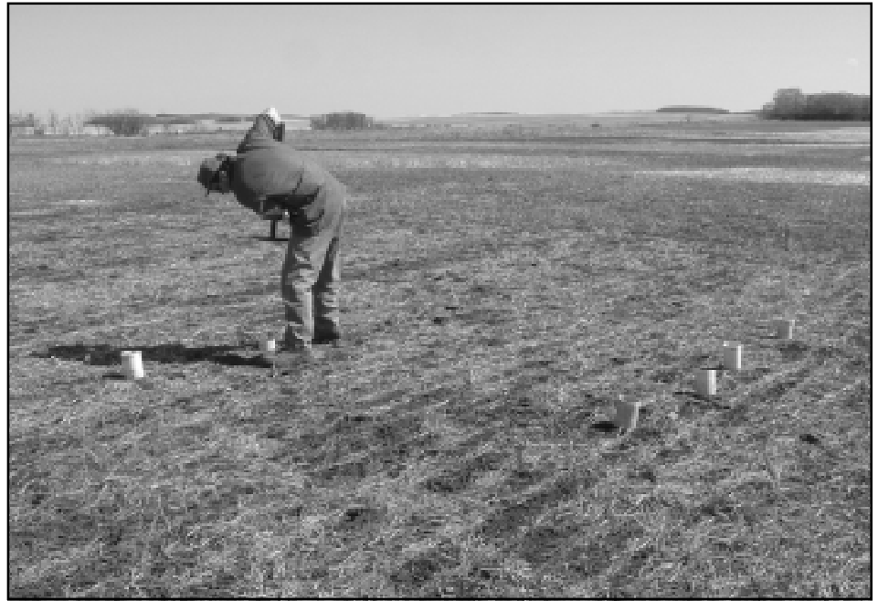
Taking soil cores to measure nutrient availability in short and long-term direct seeded fields.
